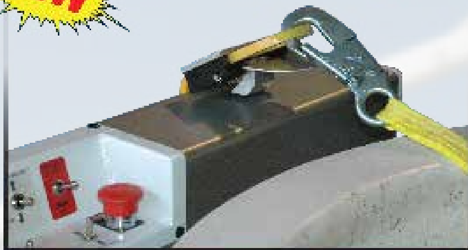
Alerts you in the operator with an audible statement: "Warning, fall protection not connected".
