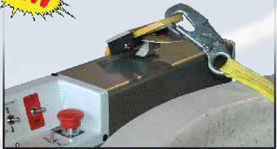
Alerts your lift operator with an audible alarm and Warning, full protection not connected.
