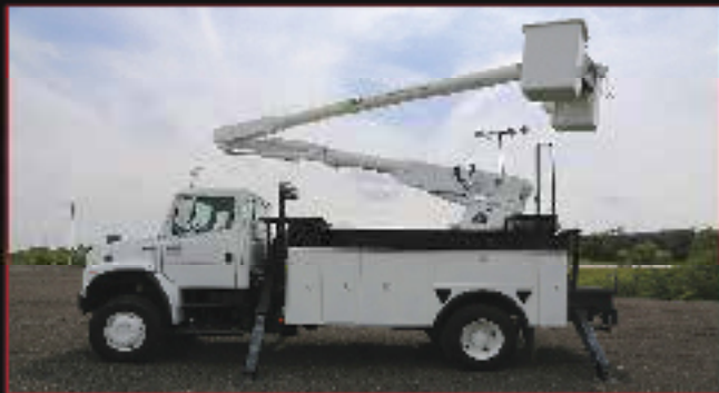
Altec AM855-2004 Freightliner FL80 4x4 Bucket Truck 2,000lb Material Handler w/Hydraulic, Ext. & Tilt, Stock # M31142CA, Odometer Miles- 03,017, CAT 3125 Diesel, 246 Horsepower @ 2,300rpm, 620lbs of Torque @ 1,450rpm, Allison Automatic Transmission, Push Button PTO w/Master Switch..... $75,250
