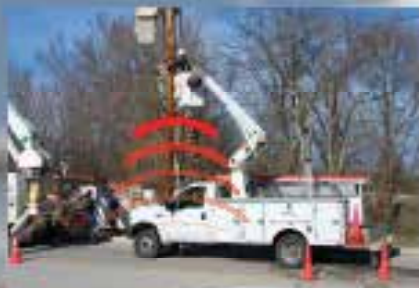
Alerts crews and bystanders when basket is descending with an audible statement, "Warning, aerial lift descending" .
