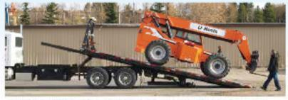
Loading construction equipment onto a transport truck is inherently hazardous, made even more so by the roll-back's steep load angle.
