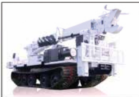
Tracked Digger Derricks
