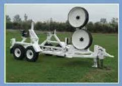
TSE 36in Bull Wheel Tensioner W/1 Disk Brake Reel Carrier
