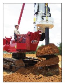
Spiradrill designs and builds hydraulic drilling rigs (truck-mounted and crawler-based units) and drilling attachments for hydraulic excavators. All are available with their lineup of custom-built dirt and rock augers or core barrel tools. Spiradrill equipment typically outdrills (depth, diameter) and offers more torque than competing products.
