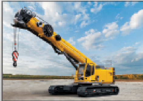
Tele-Boom Crawler Cranes
