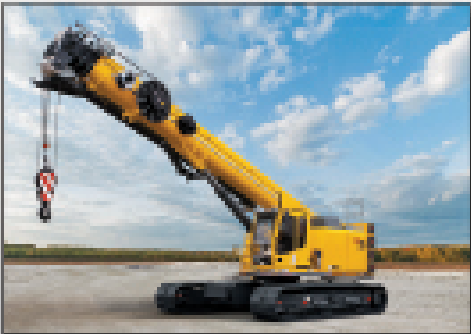
Tele-Boom Crawler Cranes
