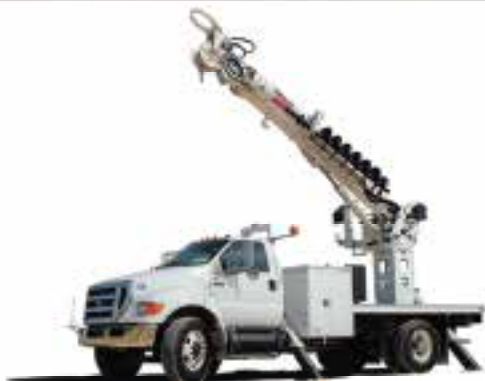
TMD DIGGER DERRICK
