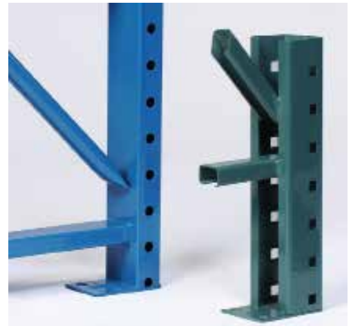
Compared to open back roll formed columns, closed tubular uprights are 44 times more torsion/twist resistant, with 250% greater frontal impact resistance and 68% greater side impact resistance.
