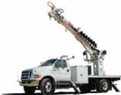
TMD DIGGER DERRICK
