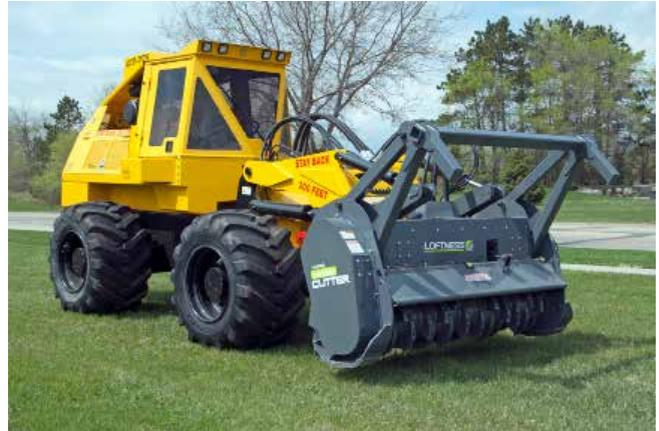
The Geo-Boy Brush Cutter Tractor from Jarraff Industries is available with various cutter head options to meet specific application needs. The Geo-Boy can be outfitted with cutter heads from multiple manufacturers.
