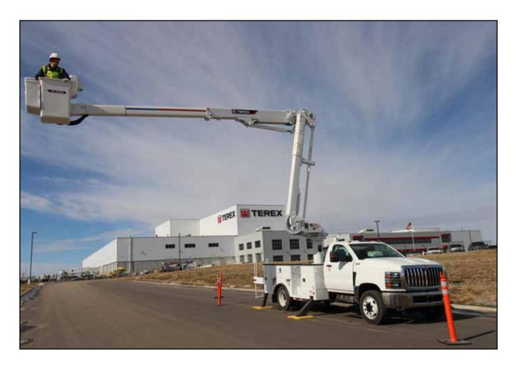
Terex Utilities also shared a new Hi-Ranger™ TL48 articulated & telescopic aerial device that is optimized for the new super duty chassis such as the Ford F600, International CV and Chevy 6500 chassis. The 53 ft. working height unit has superior jib capacity balanced with strong payload capacities to meet the needs of trouble truck applications.
