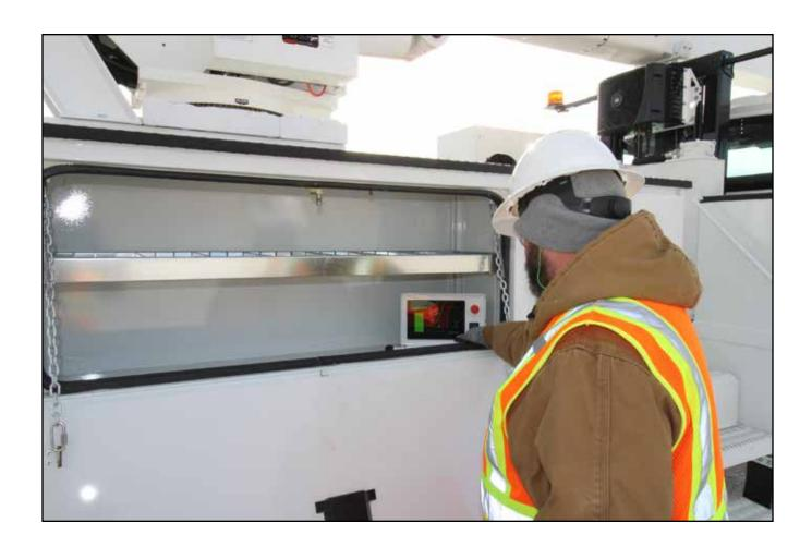
in the bucket. The system is designed to reduce the chance of an operator elevating the bucket without a lanyard attached.
