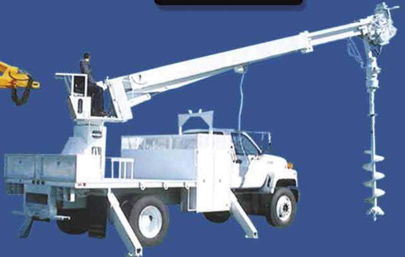
CHEVROLET Diesel Texoma TX-245B Digger Derrick
