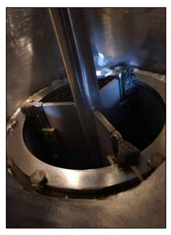
flow to the off-line chamber, opening the cover, manually removing the clogged basket, and cleaning it before refitting the basket, ensuring the seal, and tightening the fasteners.
